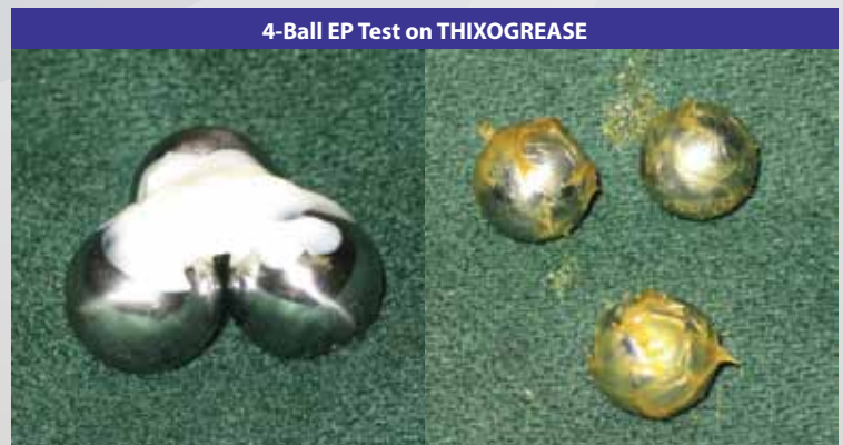
Picture 2: Steel balls coated in Thixogrease remain unmarked and moving freely in 4 ball EP wear test with 4 times the load of the previous test.
